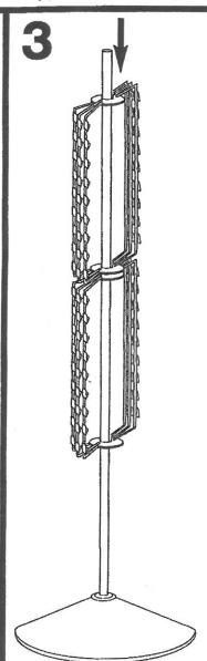
Slide second Clipper Assembly WITH CLIPS FACING DOWN over the pole and rest on top of the assembly already in place.
