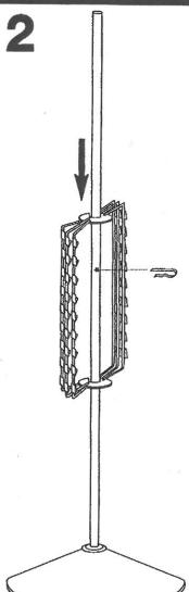
Slide first Clipper Assembly WITH CLIPS FACING DOWN over the pole until the bottom is past the punched hole. Insert the support pin and rest the top of the assembly on the support pin.
