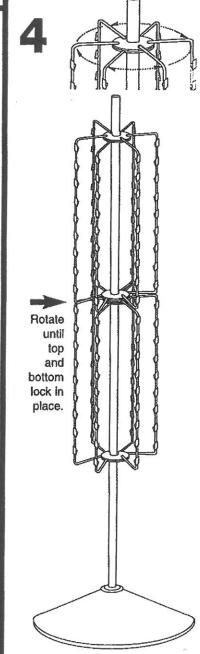
Snap open the Clipper Assemblies as shown and rotate until top and bottom assemblies line up and lock in place.
